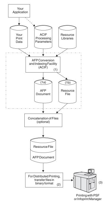
Figure 6. Using ACIF to Prepare Files for Distributed Printing
