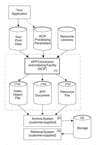
Figure 7. Using ACIF to Prepare Files for Archiving and Retrieving
