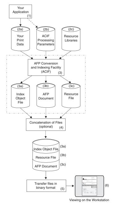
Figure 5. Using ACIF to Prepare Files for Viewing
